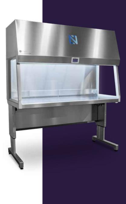
n-Safe Isotope according to EN 12469 is a Microbiological Safety Cabinet for the handling of radioactive materials n-Safe Isotope cabinets are available with a lead shielding of 1-50 mm Pb, depending on the customer's requirements. The cabinets bottom, sides and back wall can be covered with 1-50 mm lead plates, which are encapsulated in stainless steel. n-Safe Isotope cabinets also feature a slidable front on ball bearings made of 1-50 mm Pb-equivalent lead glass.
