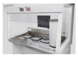
Optional H14 pre filters according to DIN12980
